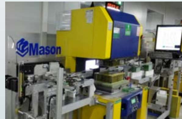
Automatic segregation test machine using 'bed of nails' - LMHV
