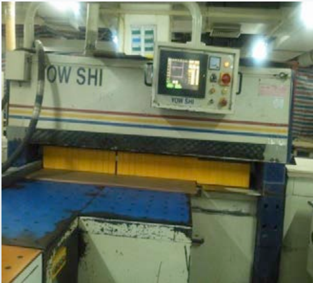
Sheet cutter – following sizes in manufacturing instruction
