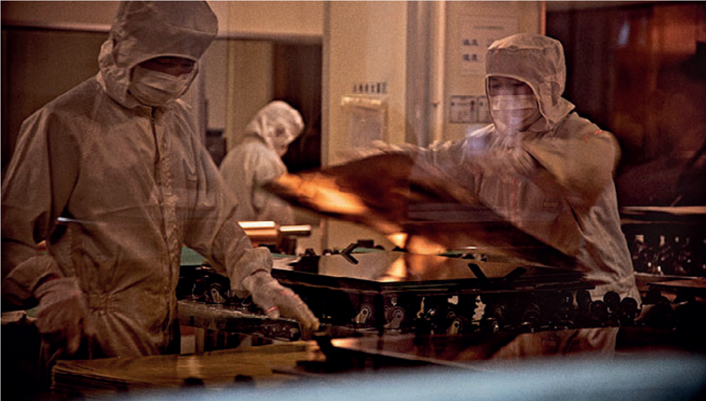
NCAB requires high standards of cleanliness, e.g. as seen here in the construction of multilayers prior to pressing.
