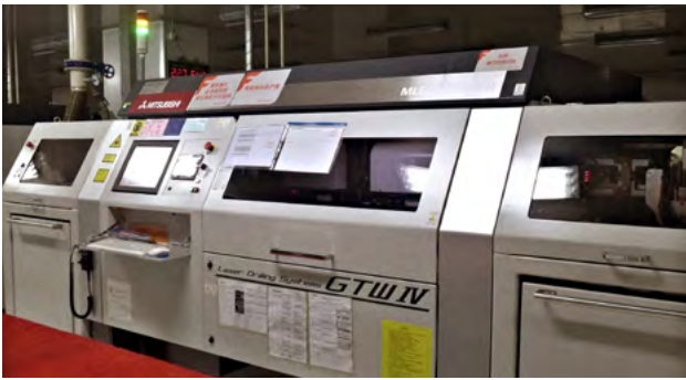
The laser drill is used in HDI production.
