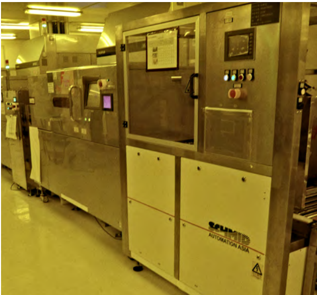
A Laser Direct Imaging (LDI) machine transfers and prints the pattern directly onto the circuit board material by means of laser beams.
