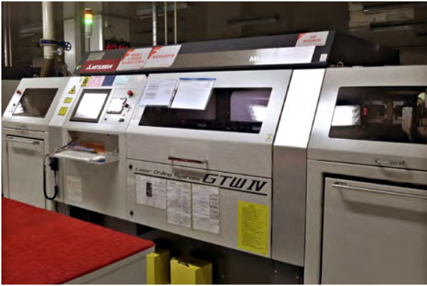
The laser drill is used in HDI production.
