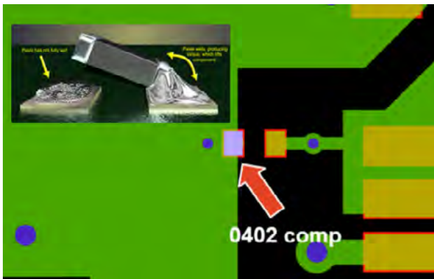
Improper SMD design affects assembly.
