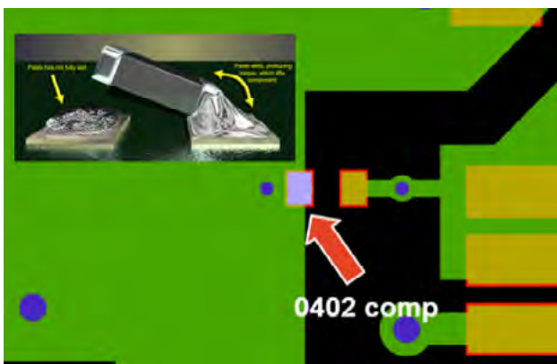
Improper SMD design affects assembly.
